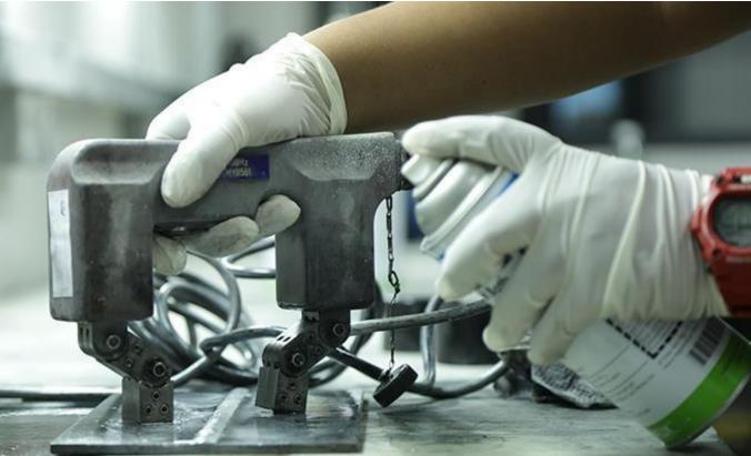
To identify a leak, ferrous particles, either dry or in a wet suspension, are applied to a part. These are attracted to an area of flux leakage and form what is known as an indication, which is evaluated to determine its nature, cause, and course of if any action.
